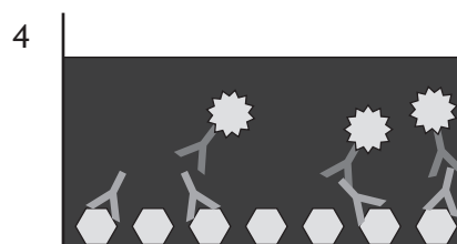
4 the plate is washed with a buffer and the substrate for the enzyme is added
